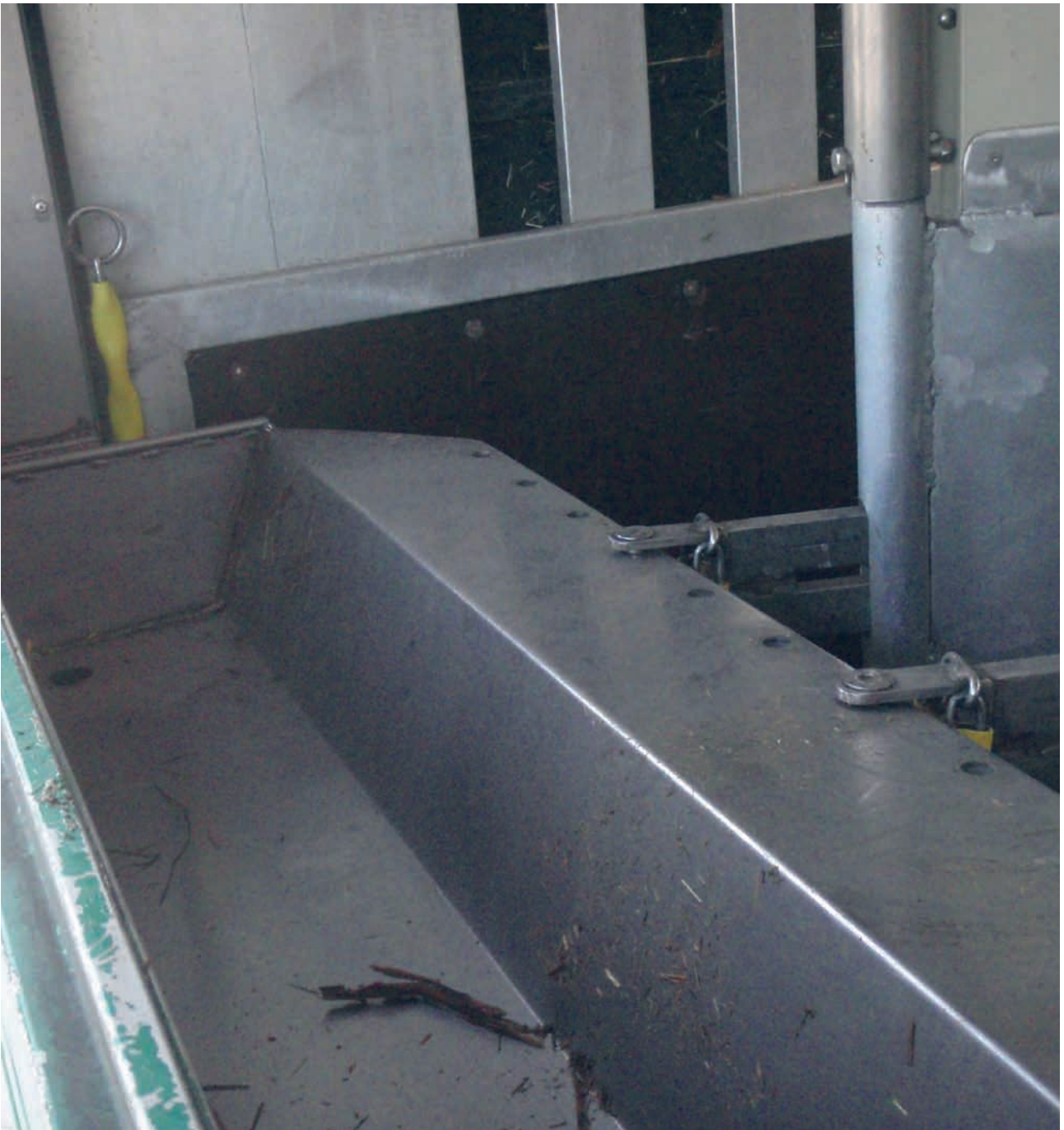
Fig. 15: Regulation compliant [Reg (EC) 1/2005], integral trough with direct connection to the water tank in the transport of horses in individual stalls. The watering trough shown here can also be used for storing feed outside of watering times.
